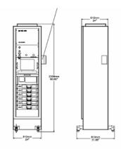
Also included is an attached control rack with unified digital control computer and color flat screen display. (left)
